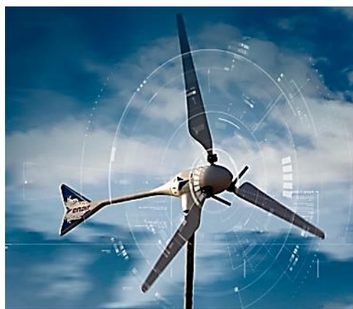
Figure 33. Horizontal wind turbine with rotor to windward. Source: Enair (n.d.)
