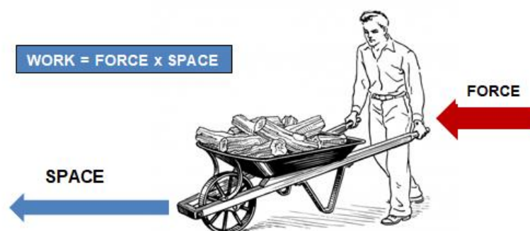
Figure 5. Force, displacement and work. Source: Adapted from Microsoft (2010)
