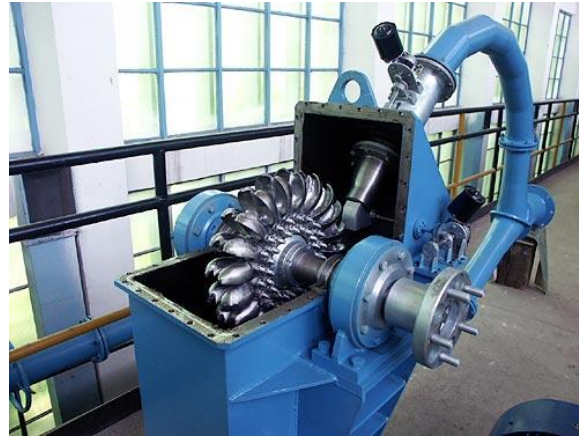
Figure 32. Pelton turbine. Source: Turbines Info (n.d.)
