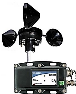
Figure 36. Anemometer with data acquisition. Source: GIS Iberica (2017)
