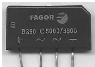
Figure 14. Single-phase rectifier. Source: Fagor (n.d.)
